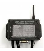
The **VC-134** radio receiver is the most widely deployed over the past couple years. It is running on an ARM processor with tons of HP. It's highly I/O dense, up to 24 outputs in a compact size and it is made of urethane potted for severe duty use. The weather and vibration are no longer an issue. One output is available as current-regulated PWM and many can be PWM without feedback and we can configure in analog and digital inputs as well.
