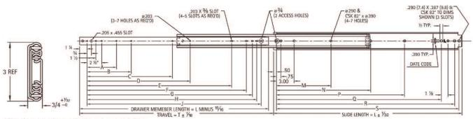
NOTE: Unless otherwise specified dimensions are in inches TOLERANCES: Fractions: Inch  $\pm 1/64^{\circ}$  Decimals: .xx  $\pm$ .010 over 18"  $\pm$ .030 .xxx  $\pm$ .005 over 18"  $\pm$ .010 over 30"  $\pm$ .015 Angles:  $\pm$  1° C' sk  $\emptyset$  + .010 - .005
