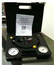
Charging kit is used to check and refill the accumulator.
