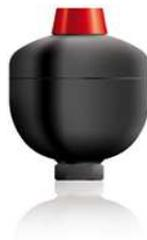
The WA accumulators are made of two hoods made of high strength steel and welded with electron beam. Those accumulators, compared to other types, have the highest energy density. This feature is due to the spherical shape of the accumulator body. Furthermore, they are maintenance free because they have been designed for high production, low cost applications, for which it is more practical and convenient to replace it than repair the equipment.
