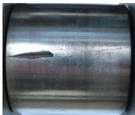
Fig. 3 - Crack on the roller
