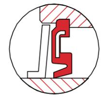
STANDARD SHIELD & RUBBER COVERED SEAL TYPE C
